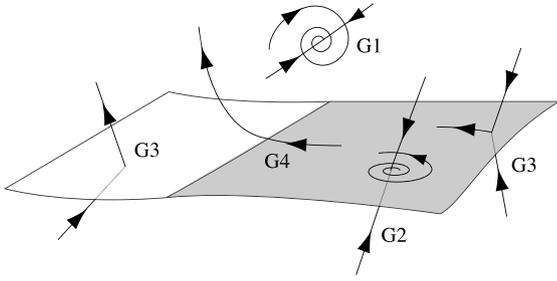
**Fig. 9.** Generic dynamics in a piecewise smooth system: G1 is an equilibrium away from  $\Sigma$ , G2 is a pseudoequilibrium, G3 is a non-sliding segment hitting  $\Sigma$  away from the boundary of sliding, G4 is a sliding segment hitting a fold transversely. The sliding region is shaded, the crossing region is unshaded.
