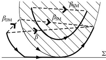
**Fig. 19.** Near a tangency, the state space is divided into two regions with different orbit topologies, depending on their intersection with  $\Sigma$ . In the hatched region the flow induces a map  $\beta = \beta_{SM}$ , while elsewhere the flow induces a map  $\beta = \beta_{SM} \circ \beta_{DM}$ .
