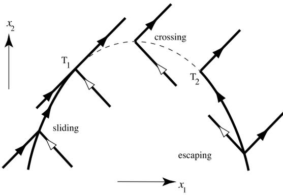
**Fig. 5.** The piecewise smooth dynamics corresponding to Fig. 4. The crossing region is dashed. A sliding segment sticks to  $\Sigma$  in the sliding and escaping regions, which are bounded by the tangency points  $T_1, T_2$ .
