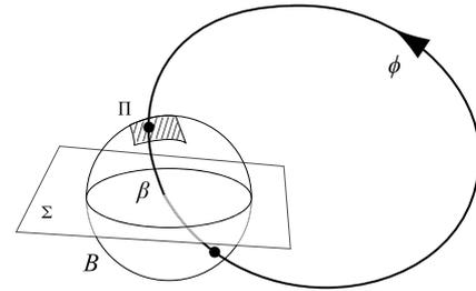
**Fig. 17.** Local analysis of a limit cycle at a discontinuity. Take a neighbourhood  $B$  of the cycle's intersection with the switching boundary  $\Sigma$ , and a Poincaré map on the section  $\Pi$ , then decompose the map into a local part  $\beta$  inside  $B$ , and a global part  $\phi$  outside.
