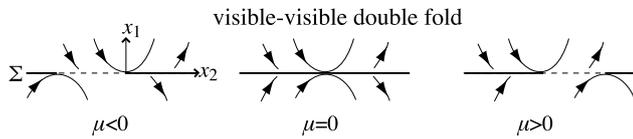
**Fig. 24.** Double tangencies and sliding regions: two folds in two dimensions. As a pair of tangencies, one each side of  $\Sigma$ , exchange ordering, a crossing region (dashed line) opens up between two visible folds, lying between sliding and escaping regions (full lines). This corresponds to (30) with the '+' signs and with  $s_1 = -s_2 = 1$ .
