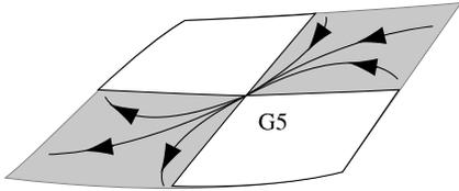
**Fig. 10.** Generic dynamics in a piecewise smooth system: G5 consists of an open region of sliding segments that hit a two-fold. Sliding/escaping regions are shaded, crossing regions are unshaded.
