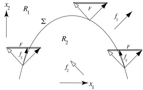
**Fig. 4.** A planar piecewise smooth vector field that switches between  $f_1$  in region  $R_1$  and  $f_2$  in region  $R_2$ . At the switching boundary  $\Sigma$  we consider the inclusion  $F$ . This gives sliding/escaping if  $F$  contains an element  $f_s$  tangent to  $\Sigma$ , and crossing otherwise.
