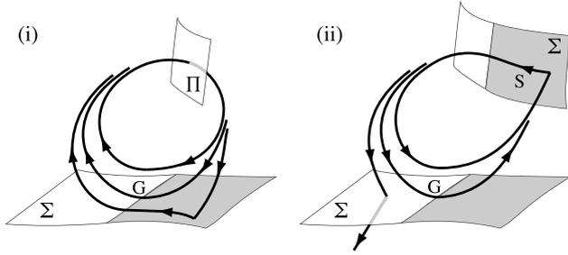
**Fig. 18.** Examples of: (i) a persistent grazing-sliding bifurcation, and (ii) a catastrophic grazing-sliding bifurcation. In (i), a cycle gains a sliding segment, and the cycle is smooth away from  $\Sigma$ , so it can be described by an invertible return map to the Poincaré section  $\Pi$ . In (ii), a cycle is abruptly destroyed, and the cycle has a sliding segment  $S$ , which lies away from the grazing point  $G$  where the bifurcation occurs, therefore it has no invertible return map.
