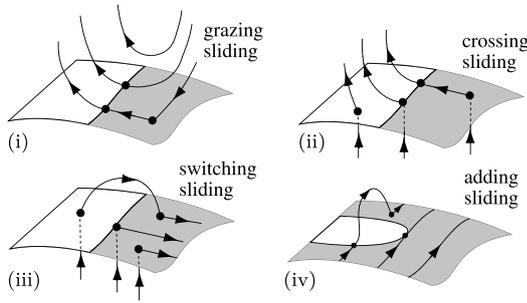
**Fig. 15.** The four sliding bifurcations. Three of these take place when a non-sliding segment hits a fold, and are called: grazing, crossing, and switching-sliding bifurcations. The fourth takes place when a sliding segment hits a cusp, and is called an adding-sliding bifurcation. A continuous change of initial condition gives a continuous change in the orbit topology, and in the orbit's interaction with the switching boundary.
