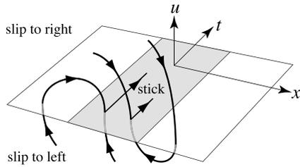
**Fig. 1.** The dry friction system (1). The friction force switches direction as  $u$  changes sign. In phase space, orbits slide along the surface  $u = 0$  (shaded) where mechanical sticking occurs. Note that ‘sliding’ here corresponds to mechanical ‘sticking’, where  $u = 0$ , as opposed to ‘slipping’, where  $u \neq 0$ .
