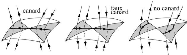
**Fig. 26.** Canards and two-folds: (i) a canard passes through a two-fold, from sliding to escaping regions; (ii) a faux canard passes from escaping to sliding regions; and (iii) a two-fold without canards. Sliding/escaping regions are shaded, crossing regions are unshaded, and the boundaries between them are folds.
