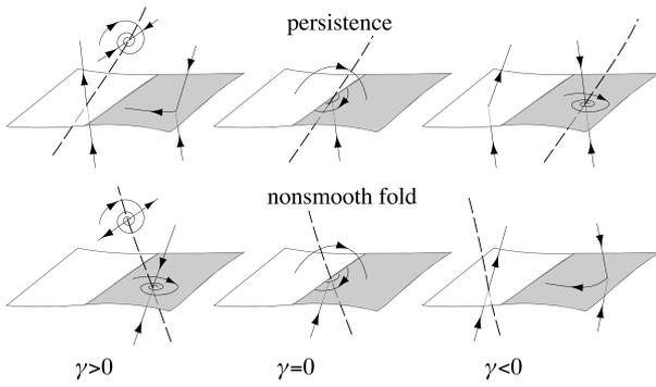
**Fig. 12.** The persistence and nonsmooth fold scenarios of boundary equilibrium bifurcations. In any number of dimensions, the functions  $f_1(\mathbf{x})$  and  $f_2(\mathbf{x})$  are linearly dependent along a one dimensional curve (dashed) given by (16). If this intersects the sliding region (shaded) then a pseudoequilibrium exists, while an equilibrium exists if  $\gamma > 0$ .
