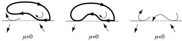
**Fig. 25.** Example of a periodic orbit destroyed in a catastrophic grazing–sliding bifurcation. As a parameter  $\mu$  changes we have: (i) a stable periodic orbit with a sliding segment, (ii) the periodic orbit grazes a visible fold at the boundary of an escaping region, (iii) no attractors remain.
