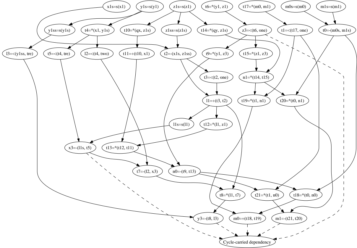
Fig. 4. High-level scheduling of the dataflow graph for the doubling step of the Tate pairing algorithm [27]. \ll is the modular left shift operator, +/- are the modular adder/subtractor, and * is the Montgomery multiplier
