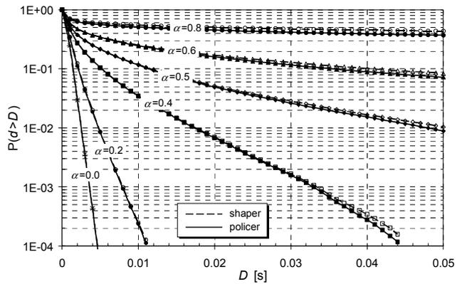
Fig. 5: Probability of exceeding delay  $D$  in a FIFO queue following a regulator ( $m_x = 2279 \text{ bit/ms}$ ,  $\sigma_x = 773.9 \text{ bit/ms}$ ,  $\tau_0 = 1 \text{ ms}$ ,  $r/m_x = 1.31$ ,  $b/\sigma_x = 18 \text{ ms}$ ).
