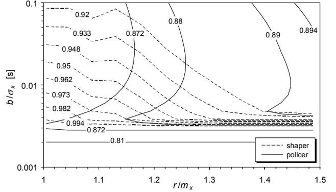
Fig. 4: Loci of the  $(r/m_x, b/\sigma_x)$  pairs for which the same  $\alpha_{OUT}$  was estimated on the traffic output by a regulator fed with fG<sub>Tr</sub> ( $\alpha_N=0.90$ ).
