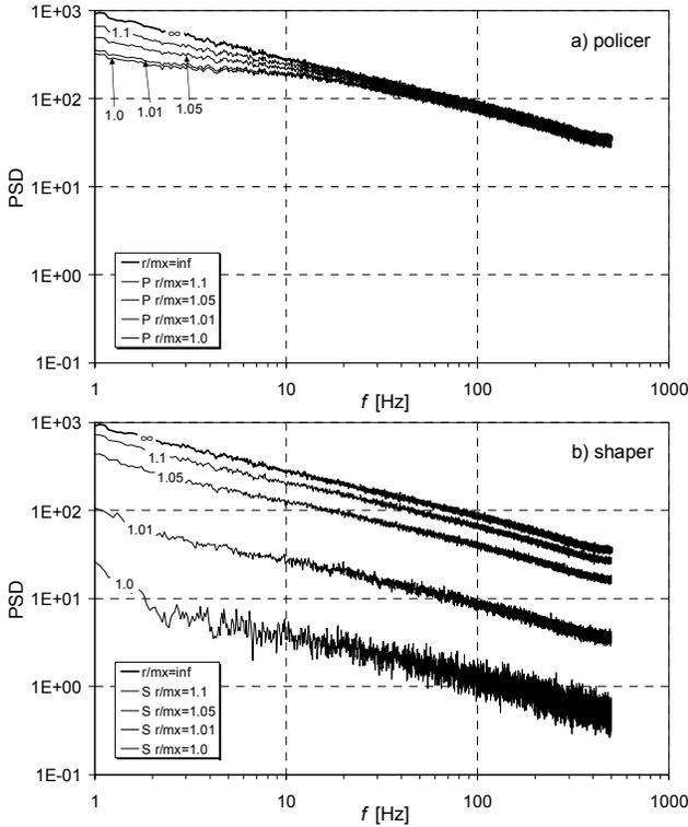
Fig. 2: PSD of traffic output by a) policer and b) shaper ( $b=14202$  bit,  $r$ ) with fG<sub>Tr</sub> input traffic ( $\alpha_N=0.50$ ,  $m_x=2.279$  kbit/ms,  $\sigma_x=773.9$  bit/ms,  $\tau_0=1$  ms).
