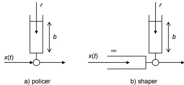
Fig. 1: Policing (a) and shaping (b) traffic regulators.
