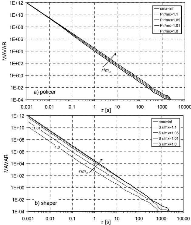
Fig. 3: MAVAR of traffic output by a) policer and b) shaper ( $b=14202$  bit,  $r$ ) with fG<sub>Tr</sub> input traffic ( $\alpha_N=0.50$ ,  $m_x=2.279$  kbit/ms,  $\sigma_x=773.9$  bit/ms,  $\tau_0=1$  ms).
