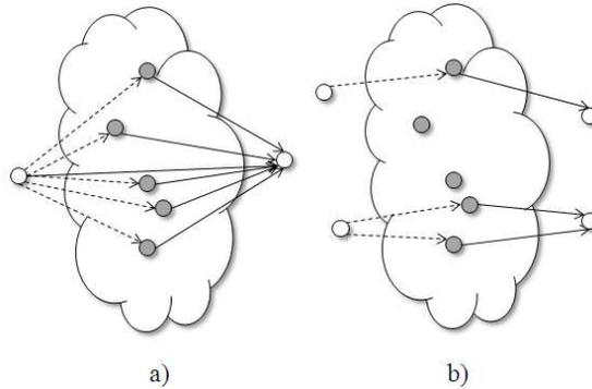
Figure 1: Cooperation and resource reuse tradeoff: a) all nodes cooperate for a single transmission, b) partial cooperation with parallel transmissions.
