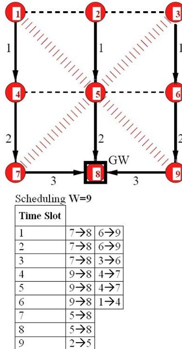
Figure 4: Solution to the GPSRP. Schedules are listed in the table
