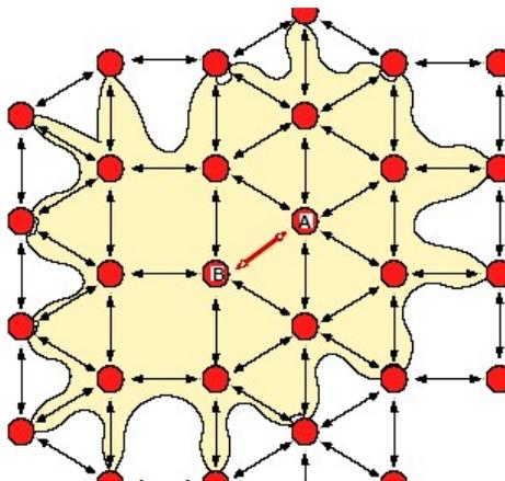
Figure 2: Interference set of the edge  $\{A,B\}$  in the binary interference model
