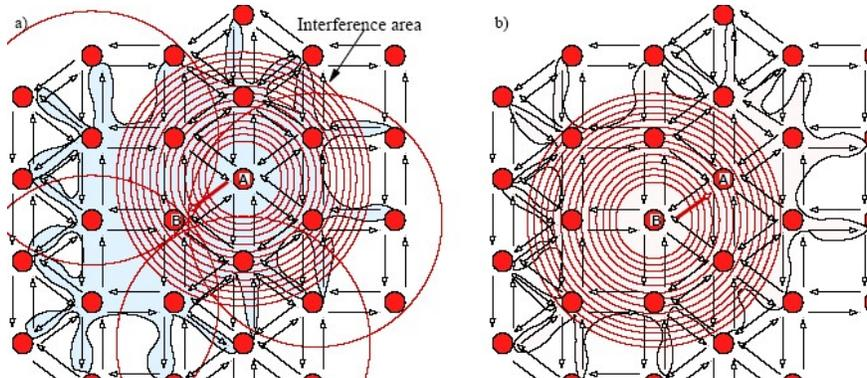
Figure 1: a) Interference set of link (A,B) b) Interference set of link (B,A)
