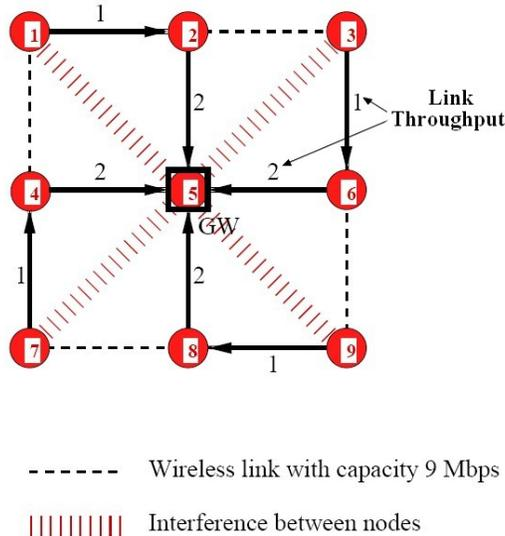
Figure 3: Solution to the GPP which considers routing. It admits no feasible schedule
