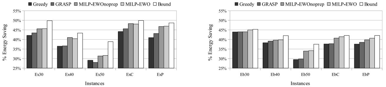
Figure 6: Comparison of the percentage of energy saving achieved by the different heuristics (Greedy, GRASP, MILP-EWO<sub>noprep</sub>, MILP-EWO) with Exodus and Ebone networks.
