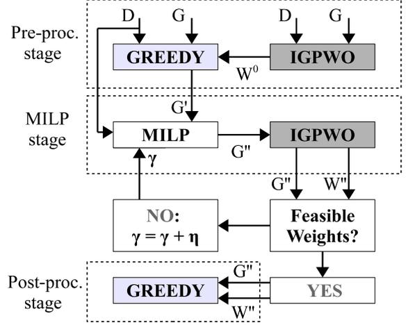
Figure 3: MILP Based Algorithm (MILP-BA) for energy saving
