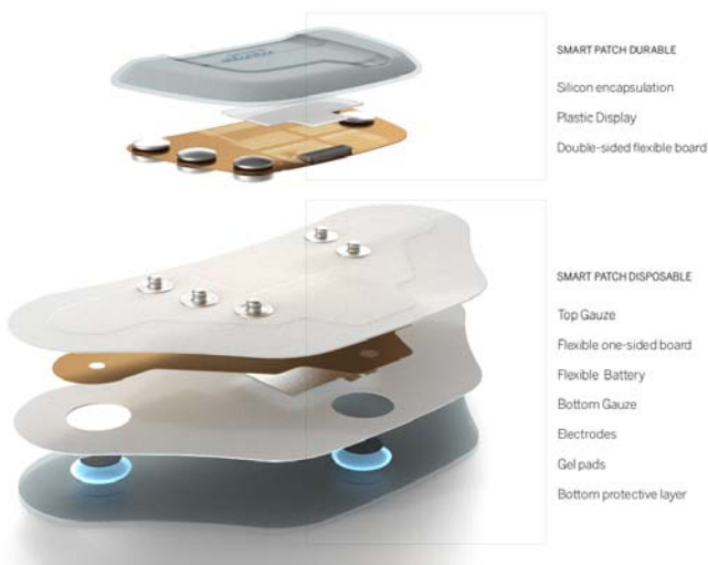
Fig. 3. Smart Patch exploded view.
