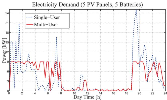
Fig. 7. Single-User and Multi-User electricity demand for low flexibility, 5 PV Panels and 5 Batteries with a two-hour tariff.
