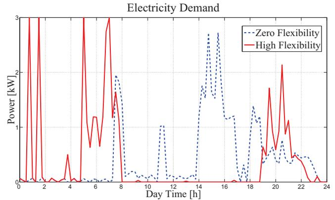
Fig. 6. Electricity demand for zero and high flexibility with a two-hour tariff.
