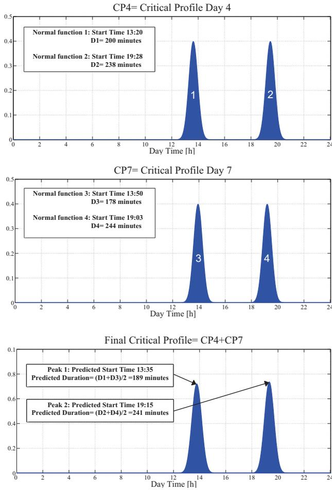
Fig. 5. Device time and duration prediction.
