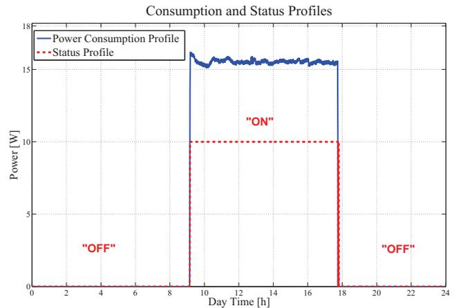
Fig. 3. Daily power consumption and status profiles for a PC monitor.
