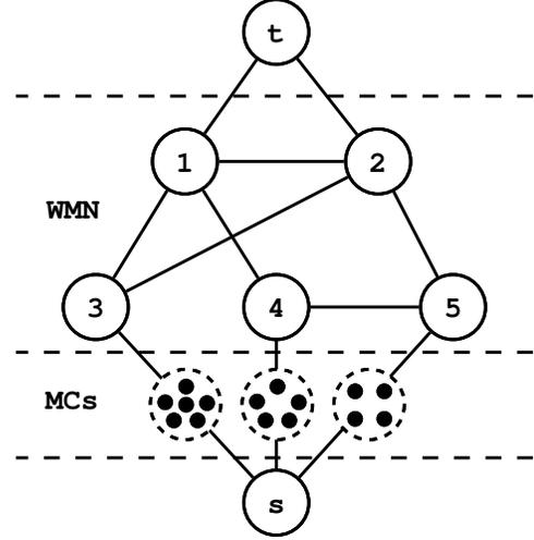
Fig. 2: Example of extended graph used by  $FeasibleSol(\tilde{x}, \tilde{y}, \tilde{d})$  to verify the feasibility of the solution obtained by selecting a new MC as winner. The black circles represent the MCs already allocated by Algorithm 3. The capacity of each fictitious arc leaving  $s$  is equal to the sum of the MCs demands inside the corresponding dashed circle.
