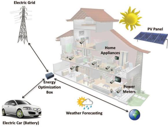
Figure 1. System architecture for a single house scenario.
