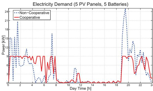
Figure 4. Cooperative and Non-Cooperative electricity demand for low flexibility, 5 PV panels and 5 batteries with a two-hour tariff.
