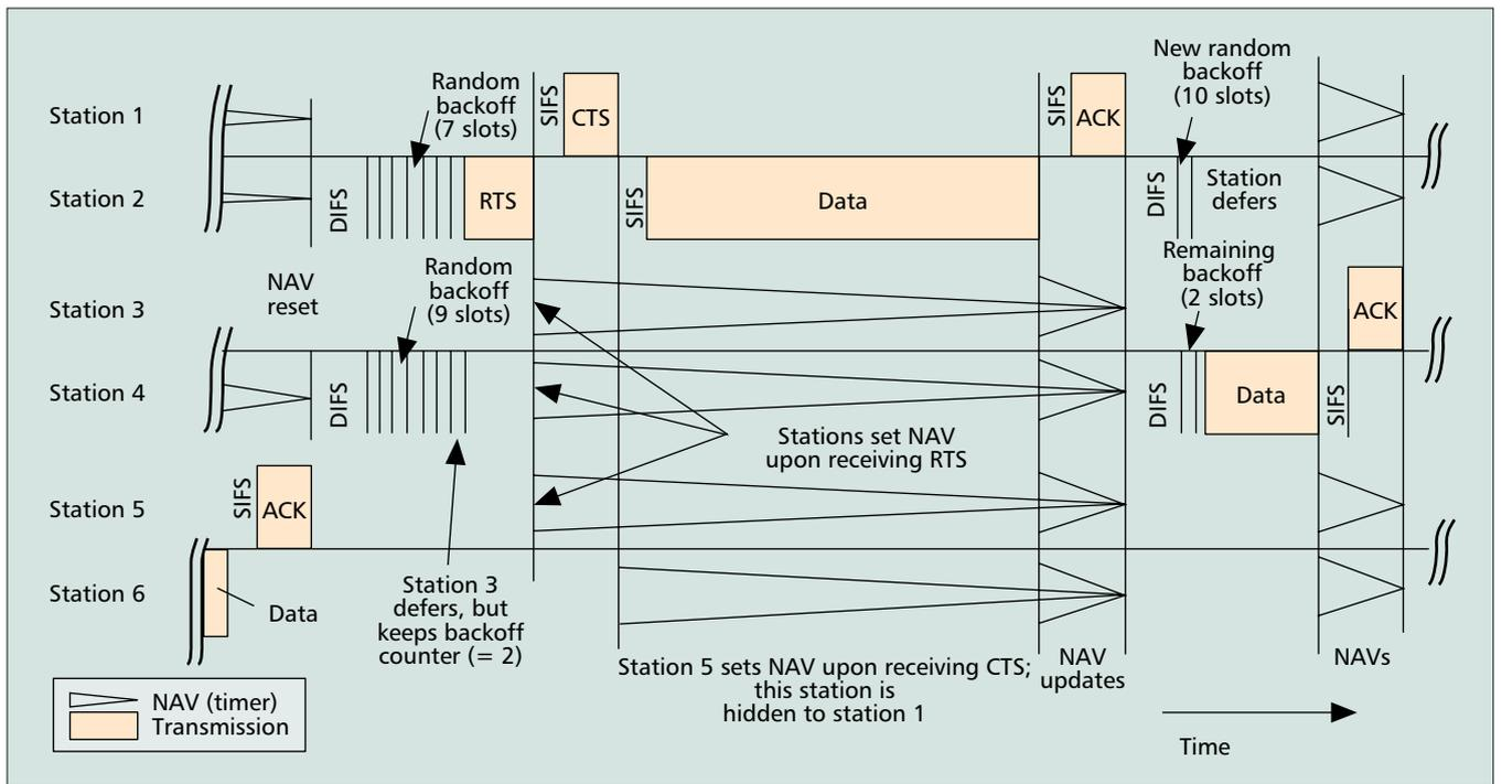
■ **Figure 2.** Timing of frame exchanges and NAV settings of the 802.11 DCF [3]. Station 6 cannot detect the RTS frame of transmitting station 2, but receives the CTS frame of station 1. Although station 6 is hidden to station 1, it refrains from medium access because of the NAV.
