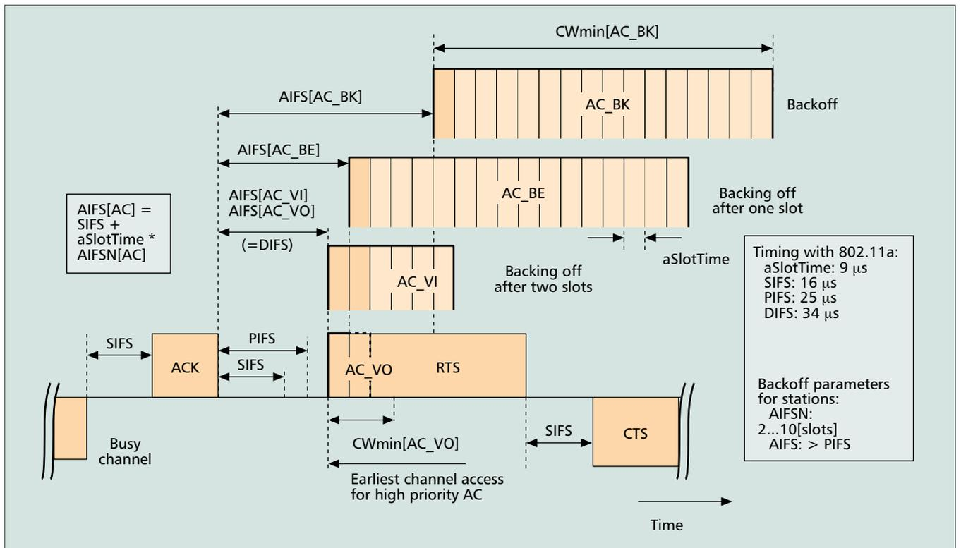
Figure 5. In EDCA, multiple backoff entities contend for medium access with different priorities in parallel [3]. The earliest possible medium access time after a busy medium is DIFS.
