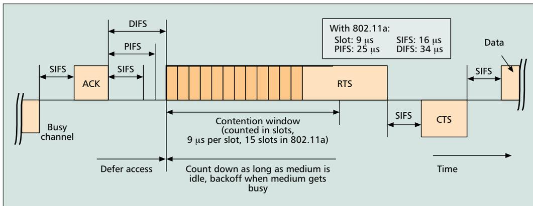
**Figure 1.** [3] Interframe spaces and backoff procedure with random contention window size. Here the transmitting station uses  $CW = CW_{min}$  (15 slots) of 802.11a, and has selected a random backoff time of 12 slots.
