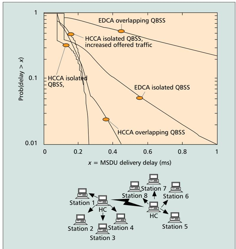
Figure 10. MSDU delivery delays for AC\_M (EDCA) and HCCA, in isolated and overlapping QBSSs. The increase of the HCCA delay in overlapping QBSSs is not under control of an HC, and therefore undesirable.
