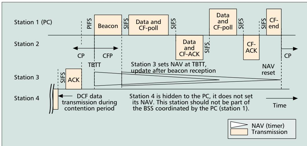
■ Figure 3. An example of PCF operation [3]. Station 1 is the PC and polls station 2. Station 3 detects the beacon frame and updates the NAV to the whole CFP. Station 3 has learned from earlier beacons that a CFP starts after the TBTT shown here.
