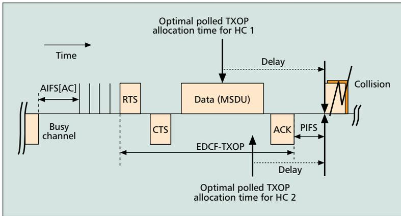
■ Figure 6. A polled TXOP allocation [3]. Any 802.11e frame exchange will not take longer than the  $TXOP_{limit}$ , which is the limit for all EDCA-TXOPs and under control of the HC.
