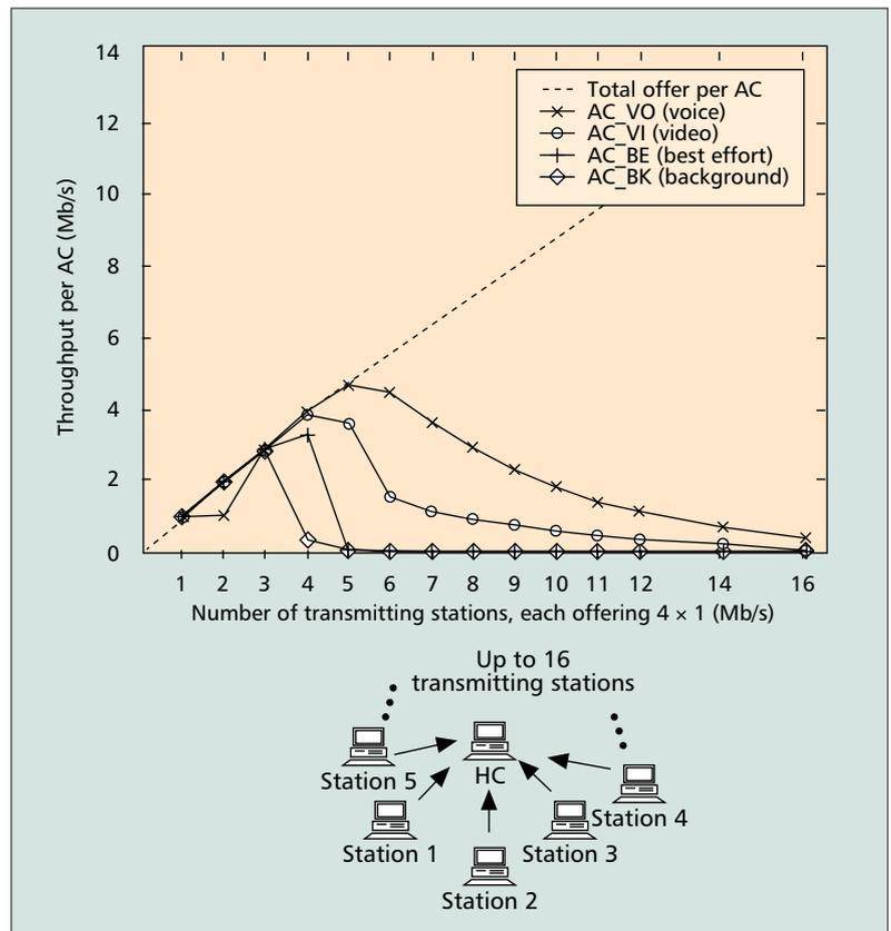
Figure 9. Throughput per AC with increasing number of stations, and constant offered traffic per station for the illustrated scenario.
