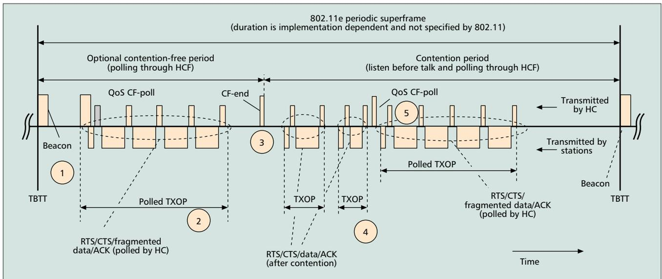
■ Figure 7. An example of an 802.11e superframe where the HC grants TXOPs in contention-free period and contention period [3]. The duration of the superframe is not specified in the standard.
