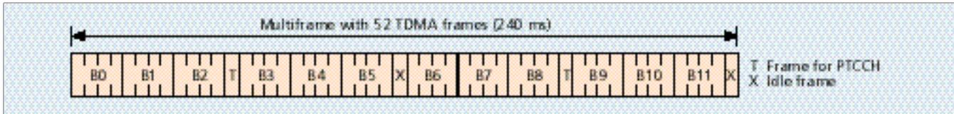
■ FIGURE 10. Multiframe structure with 52 frames.
