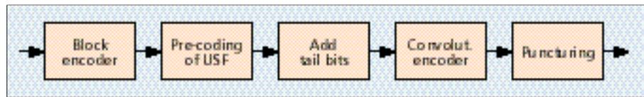
■ FIGURE 11. Encoding of GPRS data packets.
