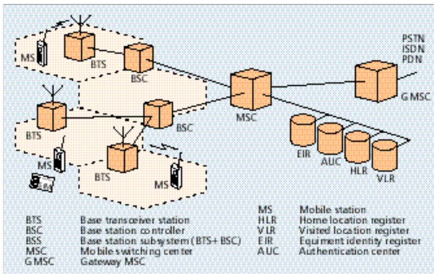
■ FIGURE 1. GSM system architecture with essential components.
