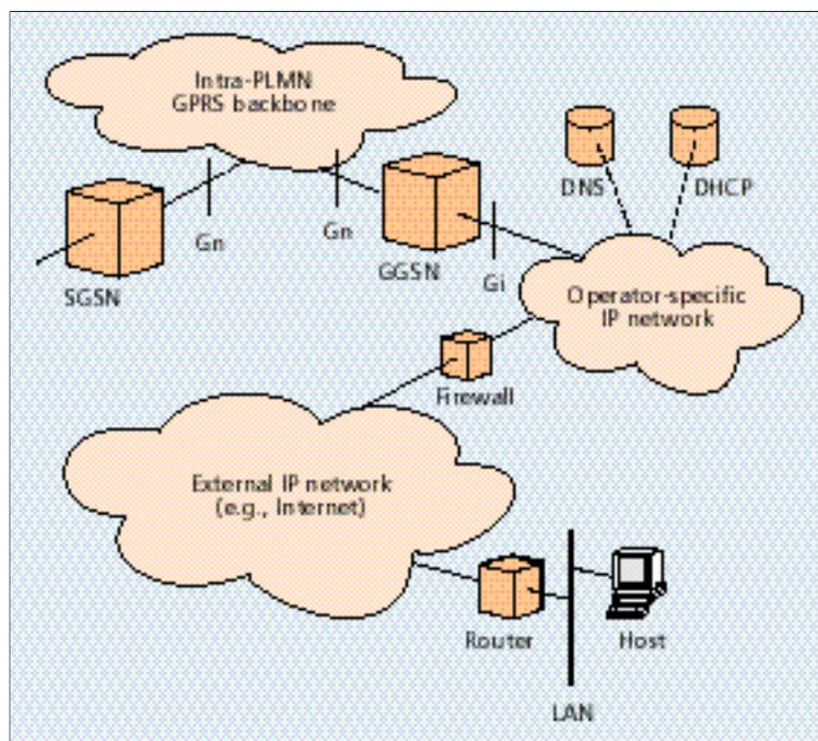
■ FIGURE 18. Example of a GPRS-Internet connection.
