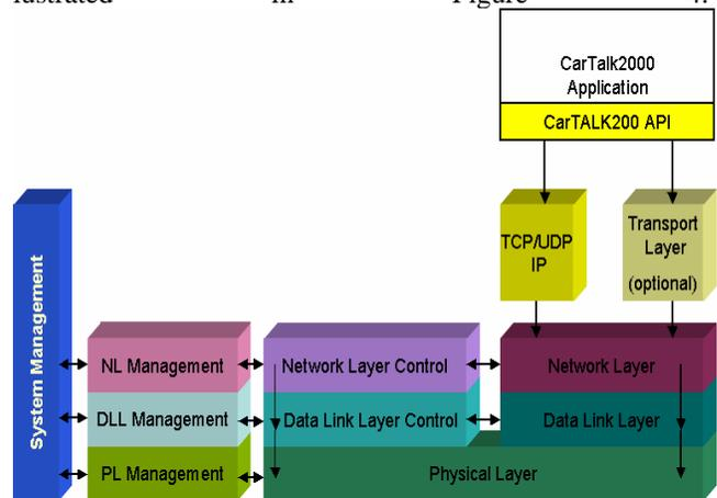
Figure 4: Protocol Architecture of the CarTALK communication system
