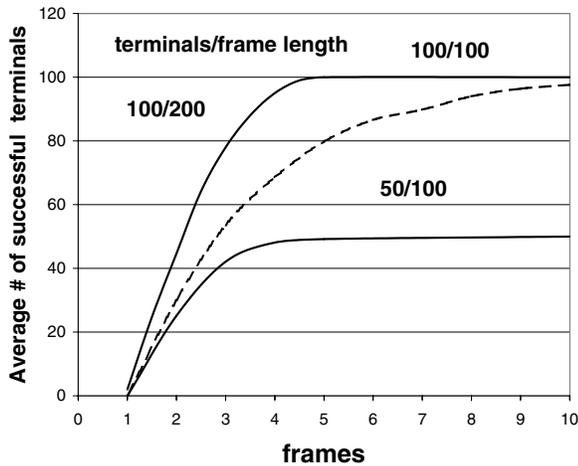
Fig. 2. Average number of terminals that have successfully accessed their slot as function of the frame number.
