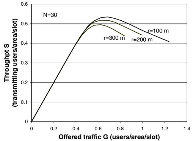
Fig. 3. The throughput of BCH channels versus the channel load for a torus surface, different coverage radii and frame size  $N = 30$ .
