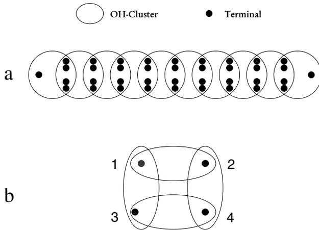
Fig. 6. Network topologies used to test the effectiveness of the multi hop broadcast service.
