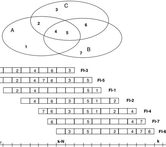
Fig. 1. Example of the FI information propagated by the terminals 1-7 in the one-hop clusters A, B, and C represented by ellipses.
