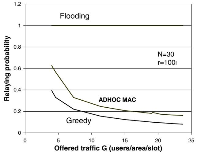
Fig. 5. Packet relaying probability versus the average number of neighbors in a square region with edge = 1Km and with coverage radius = 100m.
