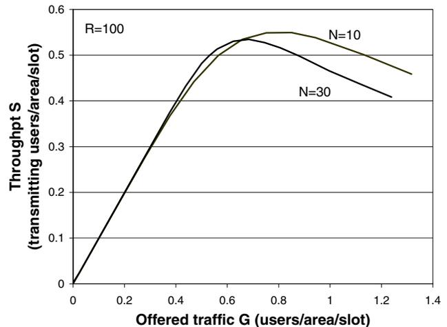
Fig. 4. The throughput of BCH channels versus the channel load for a torus surface, for different frame sizes  $N$ .
