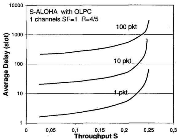
**Figure 3.** Delay versus throughput of S-ALOHA OLPC with one channel using  $SF=1$  and  $R=4/5$  when the user traffic is composed by 1, 10 and 100 packets.
