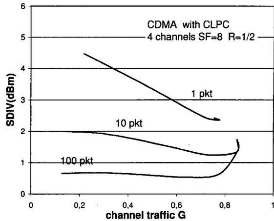
**Figure 2.** Standard deviation of the interference variation versus the channel traffic  $G$  for CDMA CLPC with four code channels using  $SF=8$  and  $R=1/2$  when the user traffic is composed by 1, 10 and 100 packets.
