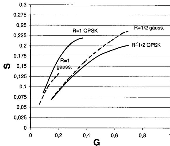
Figure 5. Throughput versus channel traffic of S-ALOHA showing the difference in results when assuming the real QPSK demodulation process and the gaussian interference model.
