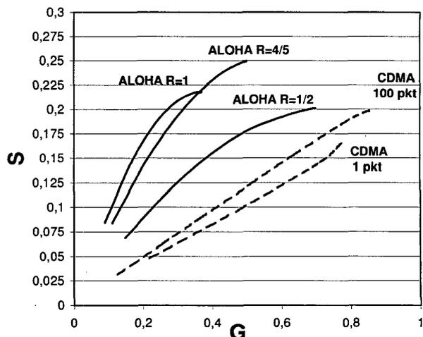
**Figure 4.** Throughput versus channel traffic of S-ALOHA and CDMA for the different cases considered.
