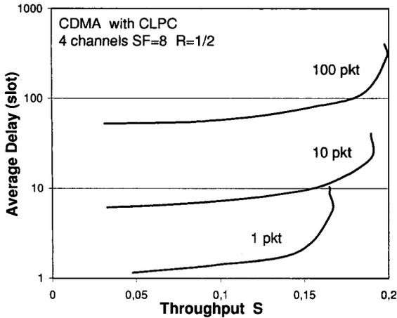
**Figure 1.** Delay versus throughput of CDMA CLPC with four code channels using  $SF=8$  and  $R=1/2$  when the user traffic is composed by 1, 10 and 100 packets.
