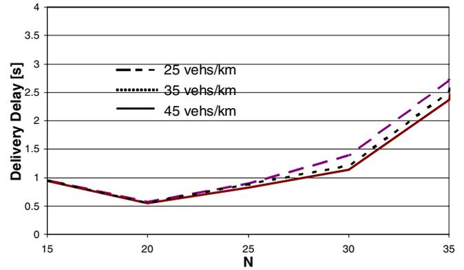
Fig. 6. Delivery Delay versus the number of slots  $N$  in the ADHOC MAC virtual frame.
