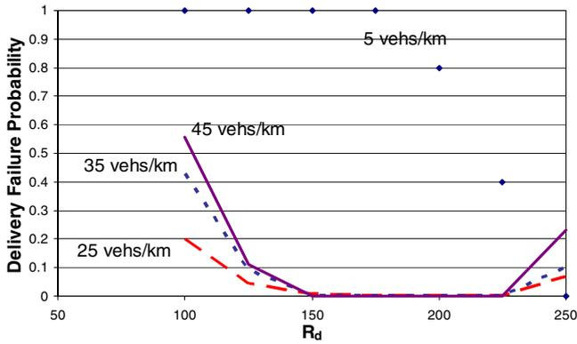
Fig. 8. ADHOC MAC: Delivery failure probability versus the decision range value for different vehicles' density.
