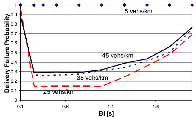
Fig. 7. Delivery Failure Probability versus the beacon interval  $BI$  in IEEE 802.11b.
