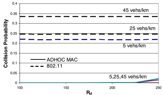
Fig. 10. The packet collision probability versus the decision range value for different vehicles' density
