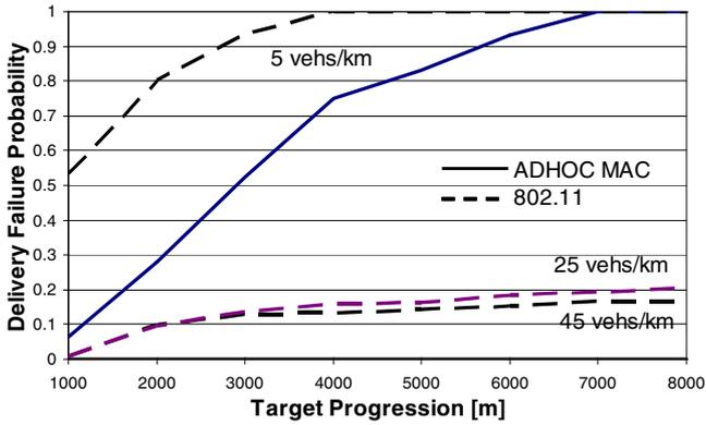
Fig. 11. Delivery failure probability versus the distance between source and destination for different vehicles' density.
