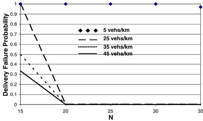
Fig. 5. Delivery Failure Probability versus the number of slots  $N$  in the ADHOC MAC virtual frame.
