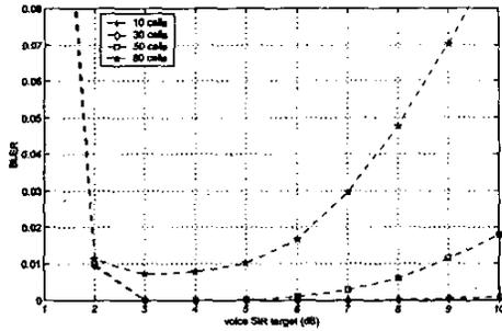
Fig. 1. Block Error Rate vs. SIR target value for different numbers of voice users per cell. No active data users.
