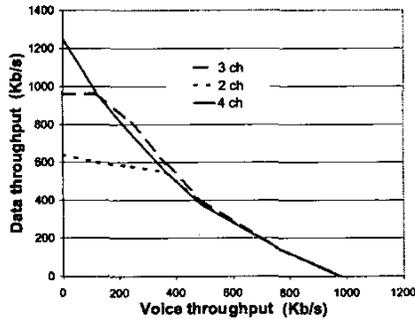
Fig. 8. Maximum throughput reached by data as function of the voice throughput, when using 2, 3, and 4 channels with SF=8 and R=1/2.
