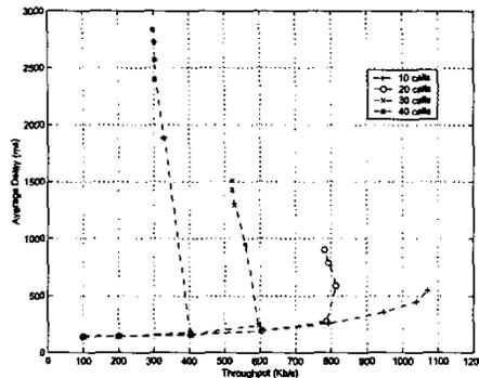
Fig. 6. Average delay vs throughput of data users with different numbers of voice users per cell when using 3 SF=8 DSCH per cell.
