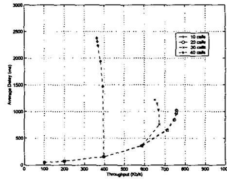
Fig. 4. Average delay vs throughput of data users with different numbers of voice users per cell.
