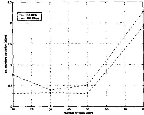
Fig. 3. Interference standard deviation vs number of voice users in the cases of no active data users and 10 active data users generating 100 Kb/s traffic per cell.
