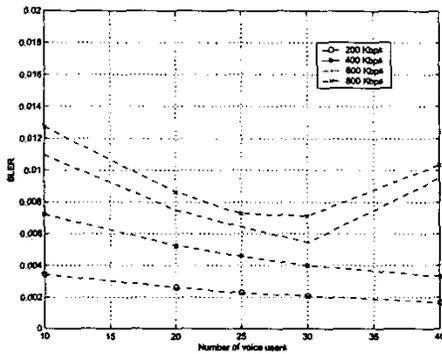
Fig. 5. BLER of voice calls vs number of voice users when varying the data offered load.
