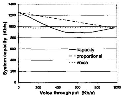
Fig. 9. System capacity as function of the voice throughput.
