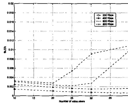
Fig. 7. BLER of voice calls vs number of voice users when varying the data offered load when using 3 SF=8 DSCH per cell.
