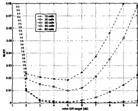
Fig. 2. Block Error Rate vs. SIR target value for different numbers of voice users per cell. 10 data users sharing a SF=4 DSCH.
