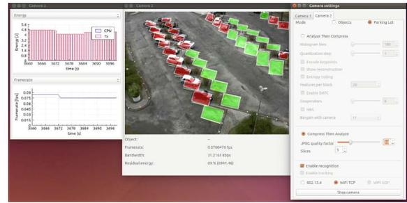
**Figure 1: The GUI used to control the VSN for the case of parking monitoring. From left to right: the real-time performance monitoring panel, the camera view and the control panel.**
