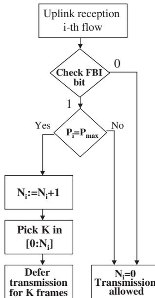
Fig. 11. Flow control scheme mobile base station side.
