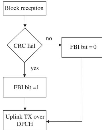
Fig. 10. Flow control scheme mobile equipment side.
