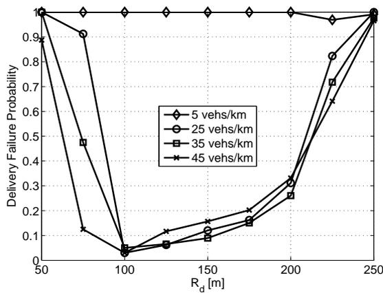
Figure 10. 802.11b: Delivery failure probability versus the decision range value for different vehicles' density.
