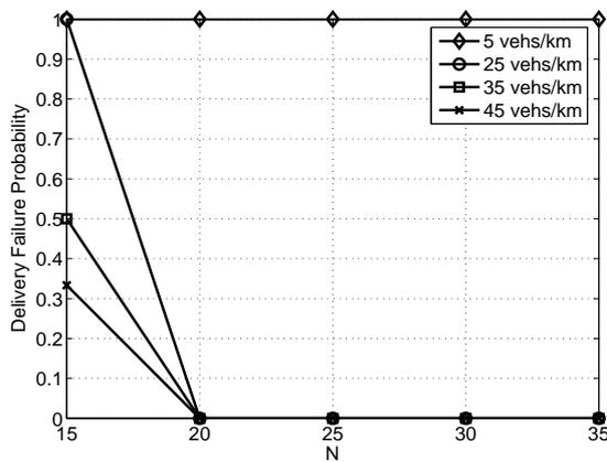
Figure 6. Delivery Failure Probability versus the number of slots  $N$  in the ADHOC MAC virtual frame.
