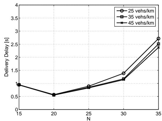
Figure 7. Delivery Delay versus the number of slots  $N$  in the ADHOC MAC virtual frame.
