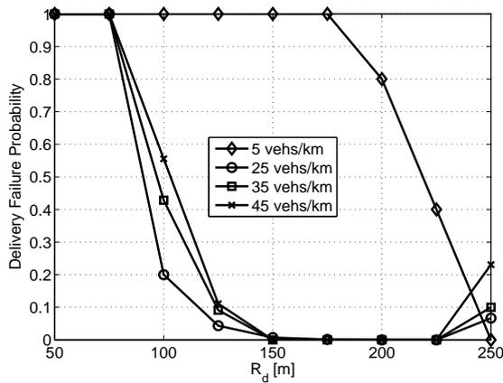
Figure 9. ADHOC MAC: Delivery failure probability versus the decision range value for different vehicles' density.
