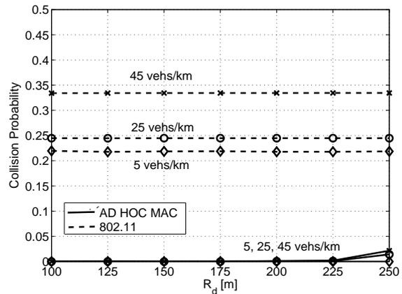
Figure 11. The packet collision probability versus the decision range value for different vehicles' density
