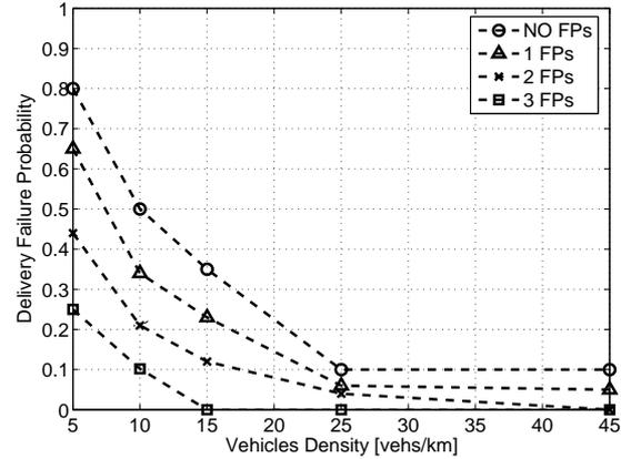
Figure 15. The delivery failure probability versus the vehicles' density for different FPs in the 802.11 case.
