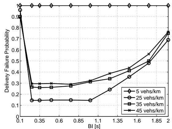
Figure 8. Delivery Failure Probability versus the beacon interval BI in IEEE 802.11b.
