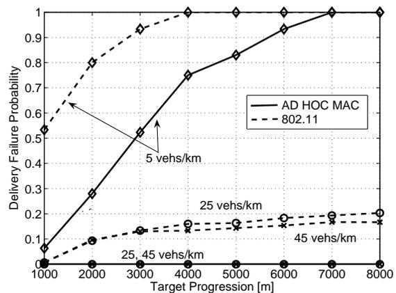
Figure 12. Delivery failure probability versus the distance between source and destination for different vehicles' density.
