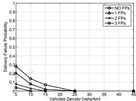
Figure 16. The delivery failure probability versus the vehicles' density for different FPs in the ADHOC MAC case.
