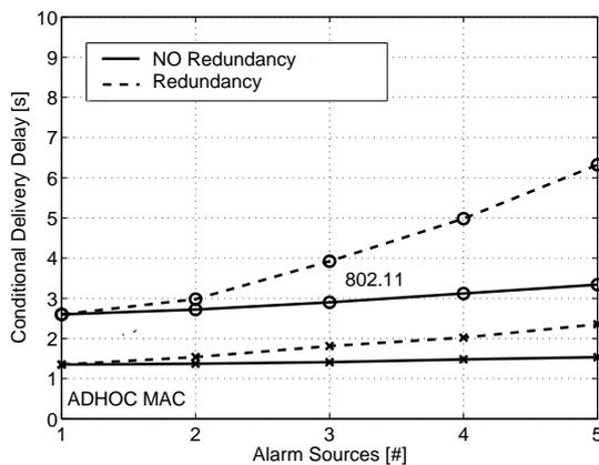
Figure 17. The delivery delay versus the number of sources when the intermediate nodes group or not the information.
