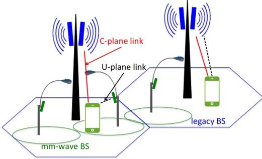
Figure 1: Dual-connectivity scenario in which C-/U-plane connections are shown.
