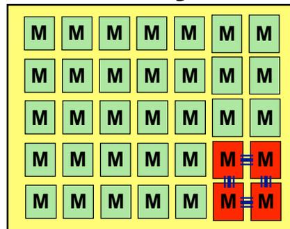
*“This design only uses 10% of the FPGA. Let’s use the macros in one corner to minimize the distance between blocks.”*
