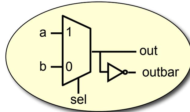
$$\text{Out} = \text{sel} \cdot a + \overline{\text{sel}} \cdot b$$
