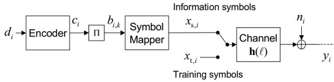
Fig. 1. Signal model for convolutionally coded system.
