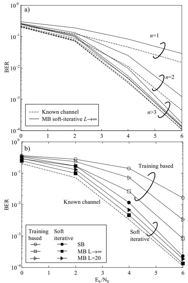
Fig. 5. BER performance for the turbo equalizer vs.  $E_b/N_0$  for varying number  $n$  of iterations (top) and at the 5th iteration (bottom).
