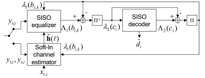
Fig. 2. Turbo receiver structure for convolutionally coded system.
