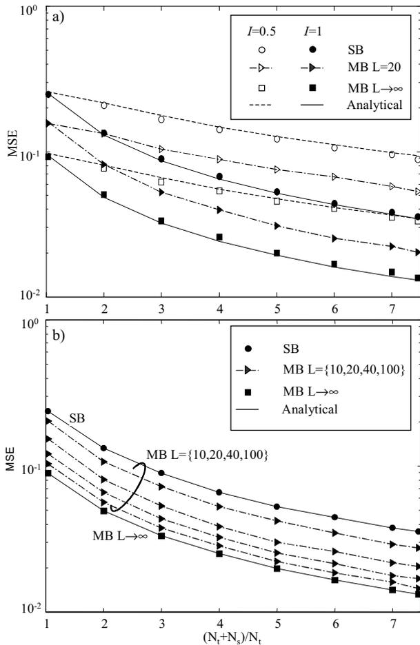
Fig. 4. MSE of the SB and MB soft iterative channel estimate for varying  $N_s$ .
