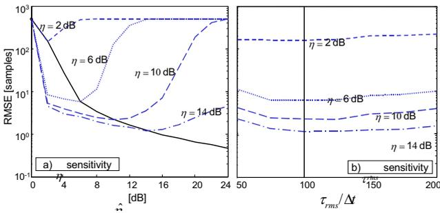
Figure 4: Sensitivity for the delay/range estimate vs. the SNR  $\hat{\eta}$  and the PDP factor  $\hat{\rho} = \exp(-\Delta t / \tau_{\text{rms}})$  used for tracking: a) RMSE vs. SNR; b) RMSE vs.  $\tau_{\text{rms}}$ . HMM parameters used:  $\eta = 2, 6, 10, 14$  dB and  $\tau_{\text{rms}} = 100\Delta t$ . RMSE is normalized by  $\Delta t$ .
