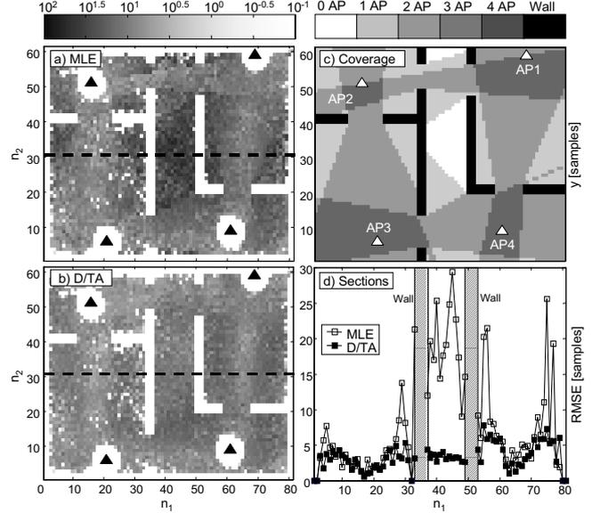
Figure 5: a-b) RMSE as a function of the spatial position for the ML estimate (a) and the D/TA (b). c) AP coverage. d) RMSE of figures (a) and (b) along the section  $n_1 = 31$  (plotted as black dashed line in figures (a) and (b)). The RMSE performance is drawn for each spatial position  $\mathbf{q} = [n_1, n_2]$  in mixed LOS/NLOS conditions. Notice that, as shown in figure (c), there is no area with coverage 4 and that a large portion lacks of coverage.
