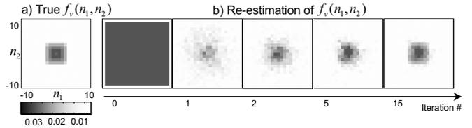
Figure 7: Re-estimation of the HMM transition probabilities  $f_v(n_1, n_2)$ : a) true probabilities (used to generate the observations); b) estimated probabilities at iteration number  $k = 0, 1, 2, 5, 15$  ( $k = 0$  is the initialization step).
