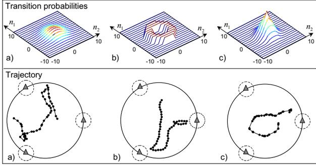
Figure 3: Examples of distribution  $f_v(n_1, n_2)$  for random 2-D driving process  $\mathbf{v}_i$ . Notice that a large  $f_v(0, 0)$  value indicates that the MS is frequently still as shown in figures a) and c).
