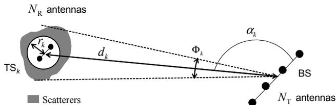
Fig. 3. Spatial structure of the downlink channel.
