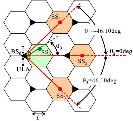
Figure 1: Cellular layout with hexagonal cells: shaded cells represent the first ring of interference for reception of the user  $SS_0$  by the base station  $BS_0$ .
