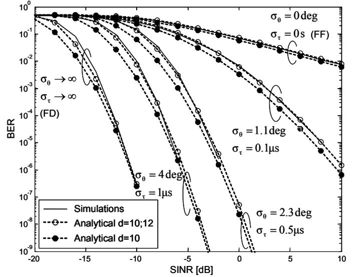
Figure 3: BER vs. SINR for a four-antenna receiver.
