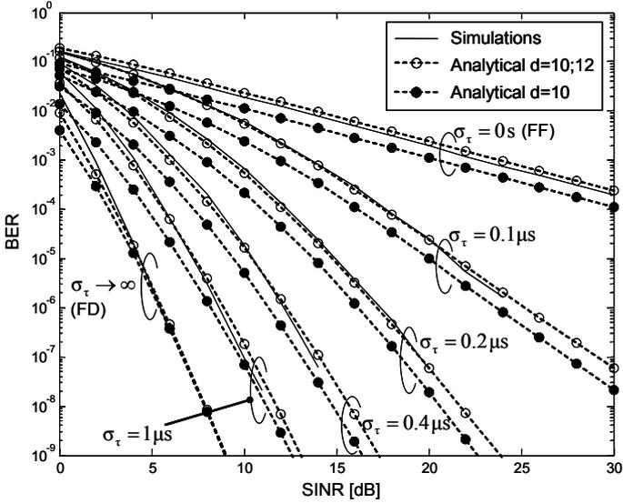
Figure 2: BER vs. SINR for a single-antenna receiver.
