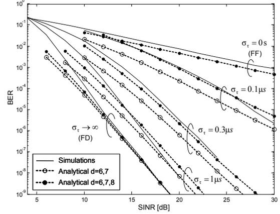
**Fig. 2.** Performance of a single-antenna WiMax system with QPSK modulation. The BER is evaluated at the output of the CC decoder.
