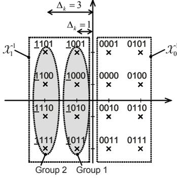
**Fig. 1.** The 16-QAM constellation with Gray's mapping. In the subset  $\mathcal{X}_1^{-1}$  there are two groups of bits with different minimum distances from the boundary of the subset  $\mathcal{X}_0^{-1}$ .
