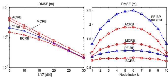
Fig. 4. Accuracy of PF-BP compared to the lower bounds vs. (left) the inverse normalized range accuracy and (right) the nodes along the 1D array.
