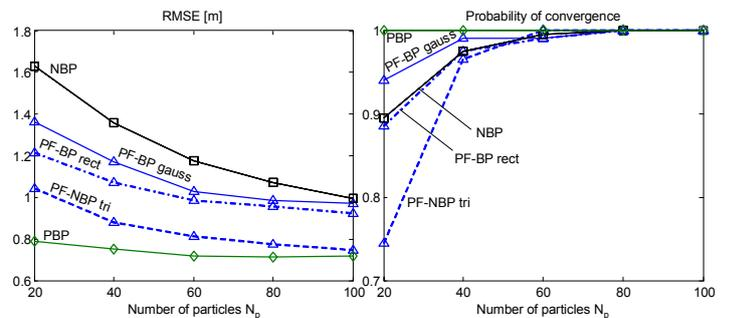
Fig. 5. Performance of BP algorithms vs the number of particles: (left) accuracy and (right) probability of convergence.
