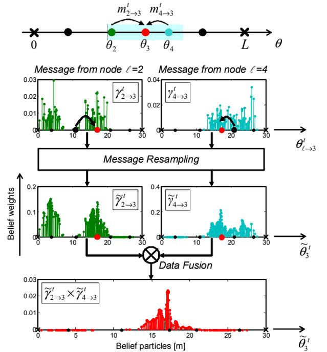
Fig. 2. Example of particle-based message fusion: at iteration  $t$ , node 3 resamples the messages from neighbors 2 and 4 over a common set of particles in order to compute the product of the two beliefs (data fusion).
