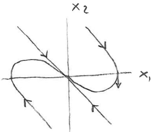
$$\left( \begin{array}{l} x(0) = \begin{vmatrix} x_1^0 \\ 0 \end{vmatrix} \rightarrow \dot{x}(0) = \begin{vmatrix} 0 \\ -x_1^0 \end{vmatrix} \\ x_1^0 > 0 \Rightarrow \dot{x}_2(0) < 0 \end{array} \right)$$
