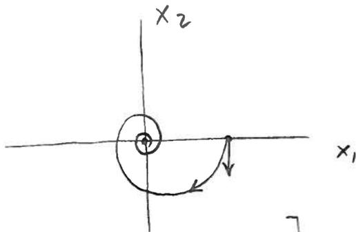
$$\left[ \begin{array}{l} x(0) = \begin{pmatrix} x_1^0 \\ 0 \end{pmatrix} \rightarrow \dot{x}(0) = \begin{pmatrix} 0 \\ p x_1^0 \end{pmatrix} \\ \text{e se } x_1^0 > 0 \Rightarrow \dot{x}_2(0) < 0 \end{array} \right]$$
