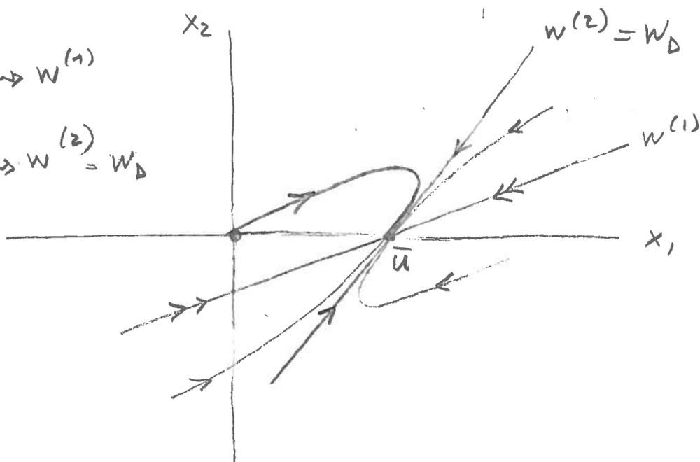
$$\text{pendenza } w^{(1)} = \frac{2}{c\left(\frac{R}{L} + \sqrt{\quad}\right)} < \frac{2}{c\left(\frac{R}{L} - \sqrt{\quad}\right)} = \text{pendenza } w^{(2)} = w_D$$
