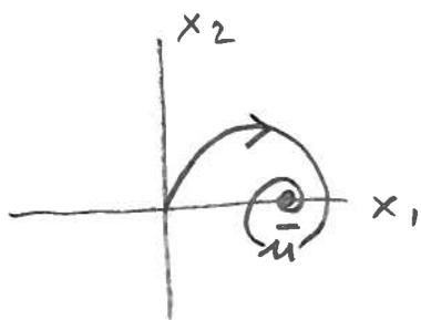
$$x(0) = \begin{pmatrix} 0 \\ 0 \end{pmatrix} \rightarrow \dot{x}(0) = \begin{pmatrix} \frac{R}{L}\bar{u} \\ \frac{1}{C}\bar{u} \end{pmatrix}$$
