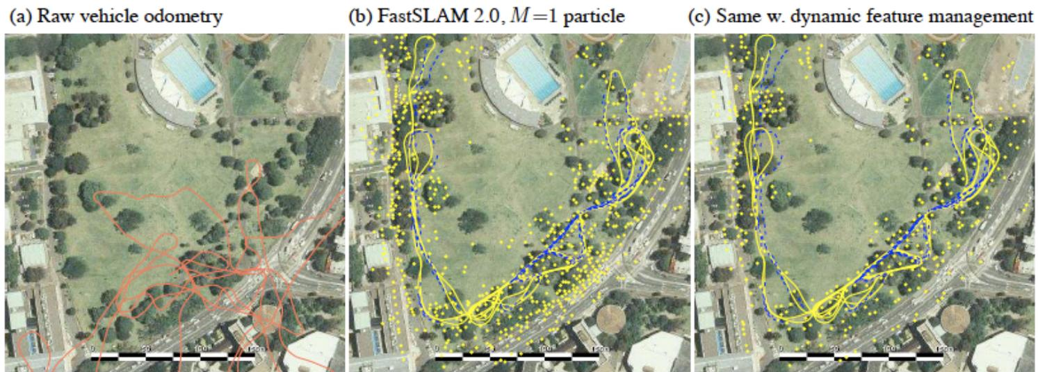
**Figure 1:** FastSLAM 2.0 applied to the Victoria Park benchmark data set using only  $M=1$  particle. The accuracy of the recovered path and the resulting map is indistinguishable from that the best EKF-style methods and the original FastSLAM algorithm with  $M=100$  particles.
