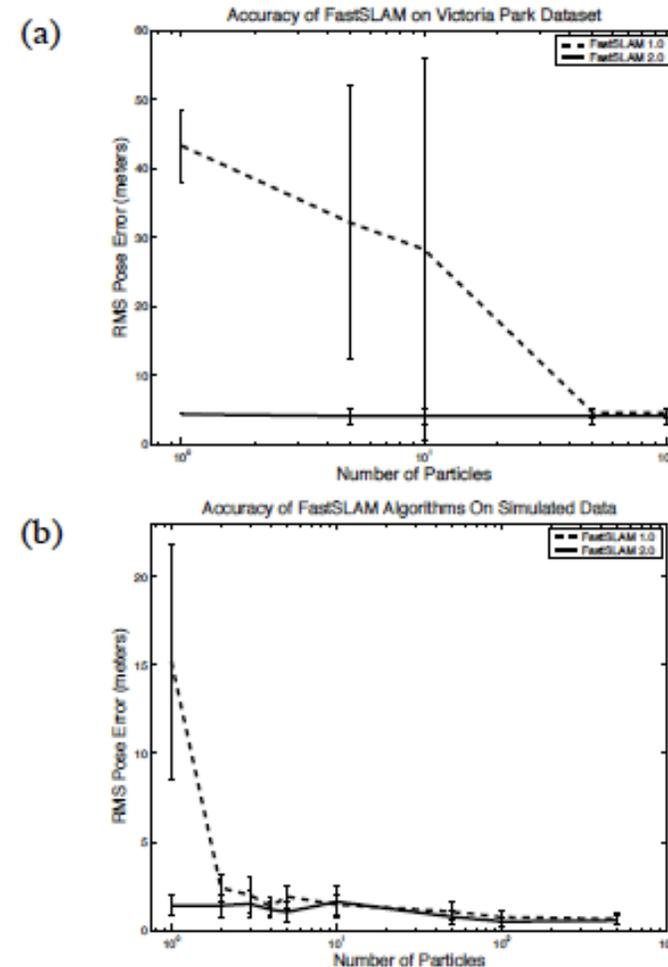
Figure 2: RMS map error for regular FastSLAM (dashed line) versus FastSLAM 2.0 (solid line) on (a) the Victoria Park data (b) simulated data. FastSLAM 2.0's results even with a single particle are excellent.
