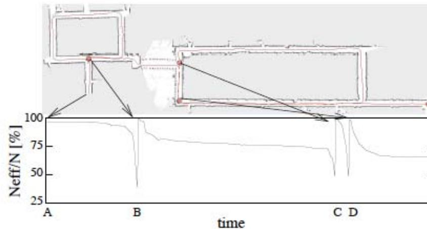
Fig. 8. The graph plots the evolution of the  $N_{\text{eff}}$  function over time during an experiment in the environment shown in the top image. At time B the robot closes the small loop. At time C and D resampling actions are carried after the robots closes the big loop.
