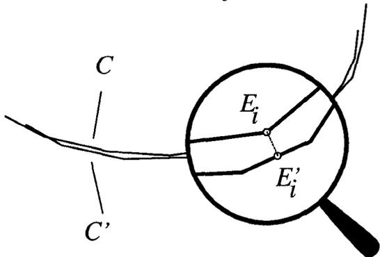
Fig. 3: 3D curve matching: evaluation of the distance between two polylines
