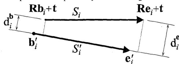
Fig. 2: evaluation of the merging cost of two straight 3D contours
