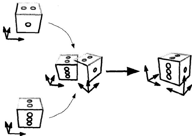
**Fig. 1: egomotion estimation through line fusion: camera motion is determined as the one that best merges the 3D contours coming from different views multi-views**
