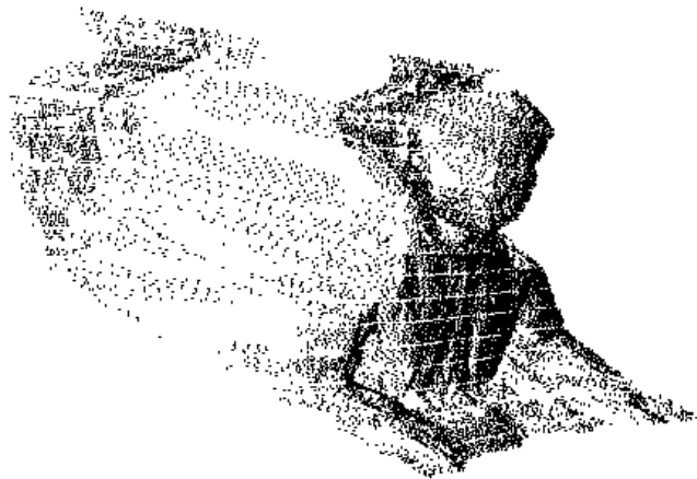
Figure 3: Example of 3D reconstruction of a teleconferencing scene from three calibrated views. From top to bottom: one of the original views; progressive refinement of the reconstructed surface, final cloud of points after outlier thresholding.
