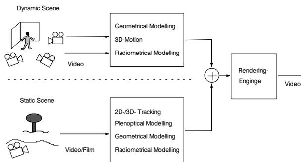
Fig. 3: Functional block diagram for the production system.
