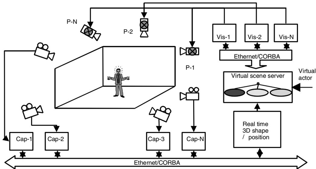
Fig. 5: Components of the real-time production and feedback system. Each camera of the multi-camera setup is connected to a server (Cap-1,...,Cap-N). A rough 3D model is created in real-time in addition to the actor head position. This information is distributed together with the virtual scene to a number of visualization units (Vis-1,...,Vis-N) that drive a data projector for the actor feedback.
