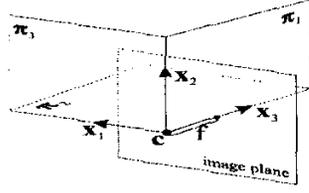
**Fig. 1.** A camera is completely defined by its axes and center, or by the three camera planes, and its focal length.
