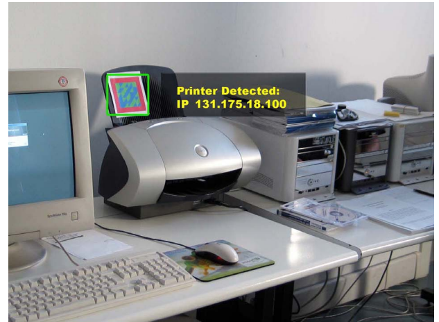
Figure 3: A tag detection in a real scene: the IP address of the printer is encoded in the tag.
