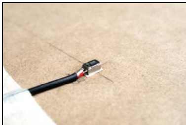
Fig. 2. Piezo-sensor BU-1771 applied to the MDF board.
