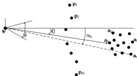
Figure 1: Notation proposed method for near-field beamshaping. The virtual source is located in  $\mathbf{s}$  and emits a beam towards the direction  $\theta$  with angular aperture  $\phi$ ; the points  $\mathbf{p}_1, \dots, \mathbf{p}_M$  denote the loudspeaker array;  $\mathbf{a}_1, \dots, \mathbf{a}_N$  are the test points.
