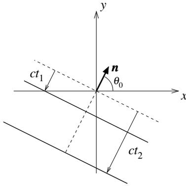
**Figure 2:** A travelling wave front for two different points in time  $t_1$  and  $t_2$ .
