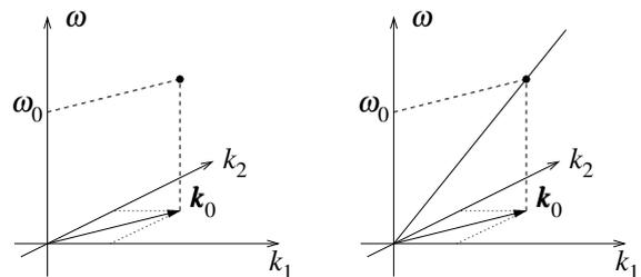
**Figure 3:** Space-time Fourier transforms of a monofrequent plane wave (left) and of a general plane wave (right).
