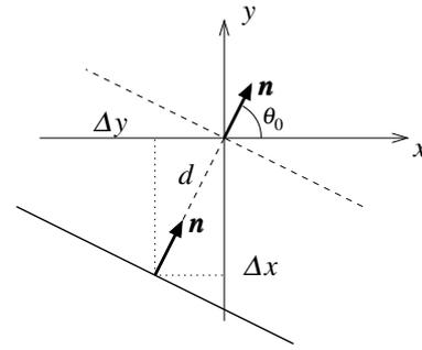
**Figure 1:** Two lines with normal vector  $\mathbf{n}$  shifted by a distance  $d$ .
